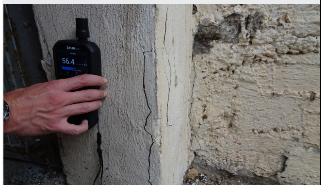
The FLIR MR277 combines thermal imaging with advanced environmental sensors to help you quickly locate, clearly identify, and easily document moisture problems.
